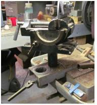
The real clever bit here is to weld a section of pipe to the plate forming the base of the vise. You can slobber weld to your heart's content and the thing will still rotate smoothly.
