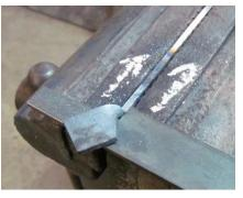
So – you now have a flag offset by about 0.125" from the spine and paralleling the spine. NORMALIZE (heat cycle) the neck & flag. The grain structure is sure to have been pooched – so correct it now and not watch the flag break off somewhere down the line.
