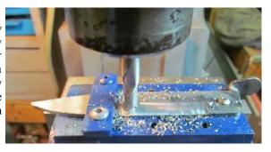
Without removing the first clamp, add another closer to the rear. You can then remove the original clamp. This way, there is never a chance of moving the blade on the mill setup. Continue milling to finish this side. Flip the blade over and reposition it to expose the unmilled side up. Re-clamp. Of course, there is a problem. The side down (just milled) is 25/1000 off of square. What to do – what to do?
