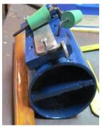
From the side you can see that there is a plate welded in the bore - it's there to stop squeezing the pipe out of round.
