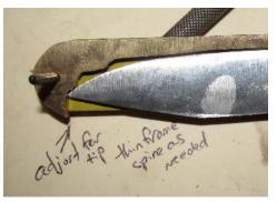
Close the blade and adjust the frame and/or blade tip as needed.
