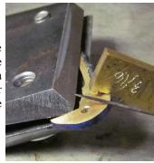
I like to use a 0.125 carbide bit on a pneumatic air die grinder (really cheap at Harbor Freight) to make a shallow depression on every other line on one side, then repeat on the other side on the alternative lines. These depressions help to lock in the chain saw file that will do the real work.
