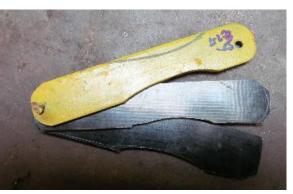
Drill the other hole. In this case, the front one is 0.154" (#22 bit). Since for me, the holes will eventually need to be the same, I drill the front, put a pin in it, clamp the sandwich again and ream out the rear. Use a #7 bit to make a funnel depression around the outside of the four holes (2 per scale). Make the depression really shallow (0.015" or so).
