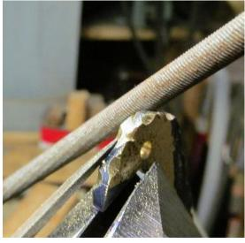
Having a rig like the one shown here makes this stuff easy. There is a well (with the long set screw) into which fits a pipe attached to the base of a small vise. This means you can change the angle relative to the floor by  $360^{\circ}$ . The vise allows a  $90^{\circ}$  rotation perpendicular to the floor. The jig to hold the frame is two pieces of plate bolted together with the shorter one with a 1/4" piece of square stock at the base, therefore "pinching" the frame.
