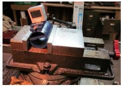
Now – toss that puppy on the mill and plop a digital protractor on the blade (having zeroed it on the vise, of course)
