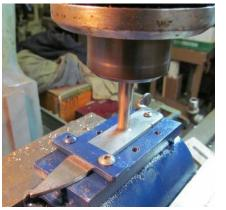
It's then etch-a-sketch time. Carefully approach the perpendicular line and plow through to the edge – and there is your plunge cut. Mill towards the tip until you get close to the clamp. Take as many passes are needed to push the bevel to the designed termination point (0.375" from the spine). Then STOP milling.
