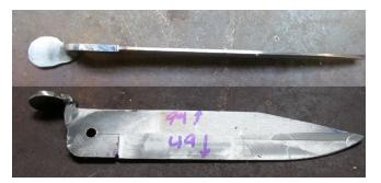
Heat treat the blade being sure to normalize the entire blade (do the neck again to be sure). Using O1 as a steel, satanite as an anti-scale, a reducing flame of an oxypropane torch, and the usual toaster oven to temper seems to work just fine. Of course, austempering would be better but for one blade....
