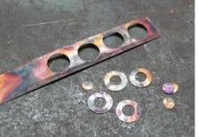
It's now time to assemble. Slip cutler rivets through the bottommost scale (good idea is to wax them a bit), drop a washer over the pivot, then blade and the other washer. Mix epoxy as described above and slip the last scale in place. Tap the rivets as the epoxy sets up but do not remove them.
