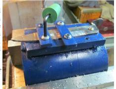
Slip a 25/1000 copper shim under the edgeto-be and repeat the milling operation described above. When done, run a #22 bit through the hole (up from #27 which is right for the 6-32 screw – see I did tell you why I bumped the 1/8" up with a #27). Now why the #22 – just wait.
