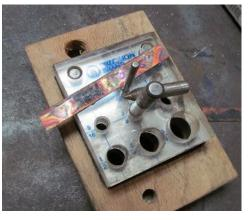
The game is to slide the strip with the 3/16" holes under the 3/8" port and feel for the hole with the pointed tool. When you feel it, the strip will align nicely with the port. Insert the 3/8" punch and whack, you've got a washer.
