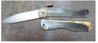
Clamp as before and make sure that the epoxy completely fills the depressions in the vine filing. Cutler rivets were chosen solely on the basis of being the only small bore brass tubing in my shop on build day. It would be better to just hit an ACE hardware store and buy a foot of appropriate tubing.
